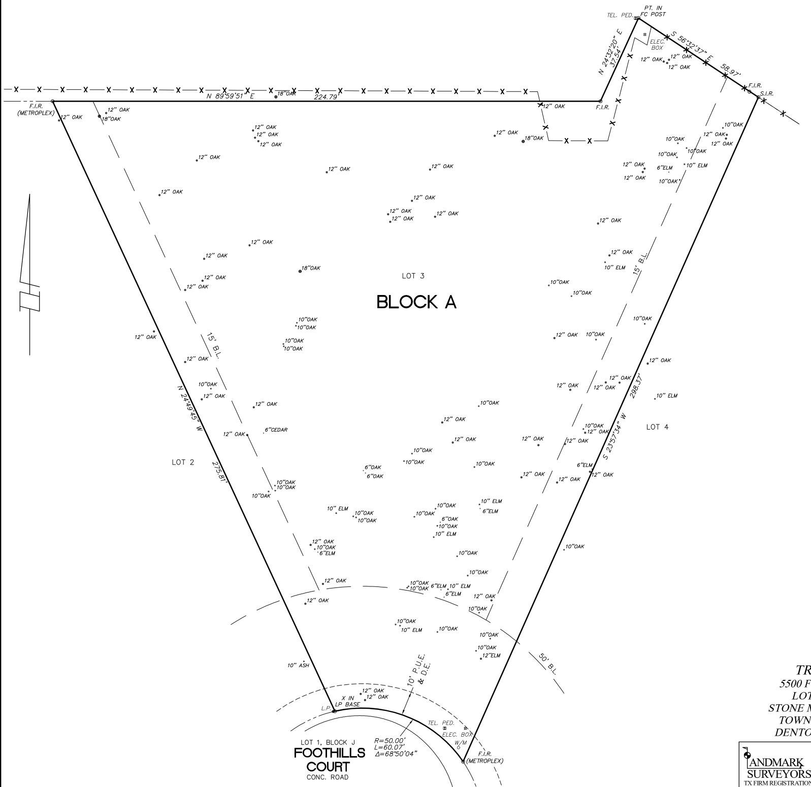
Basis of Bearing is the State Plane Coordinate System, Texas North Central Zone (4202), North American Datum of 1983, as determined from GPS observations.
